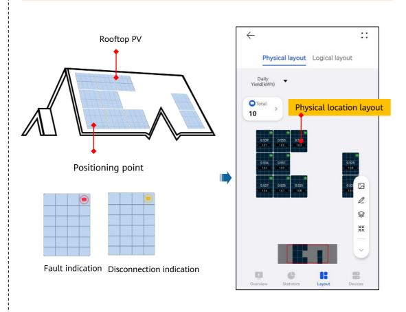
Step 1 After determining the installation position of an optimizer, remove the SN label from the optimizer and attach it to the physical layout template.
